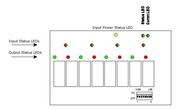
Figure 3. The board layout of the FN485-4xSH
