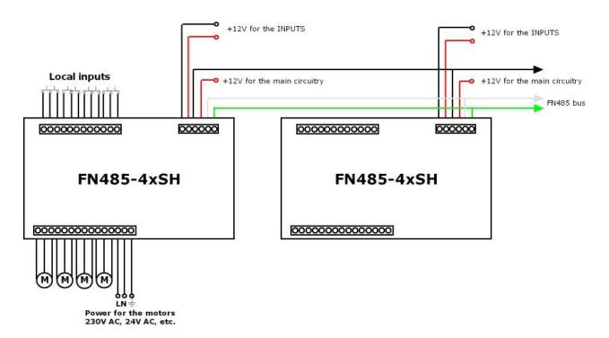
Figure 4. Connection Diagram
